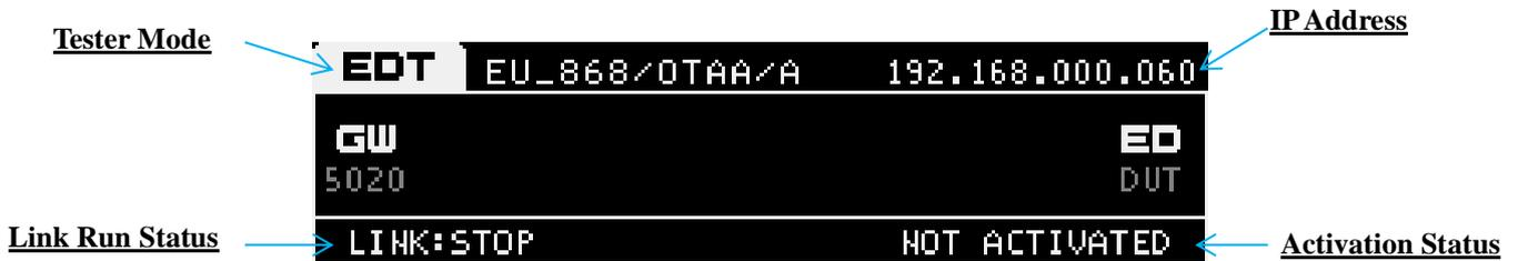
Fig A.3 RWC5020M Screen in IDLE state
