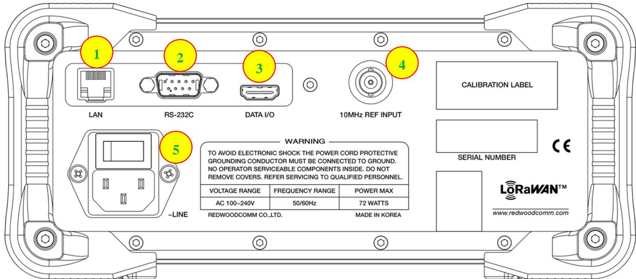
Fig 2.2 RWC5020A/B Rear Panel View
